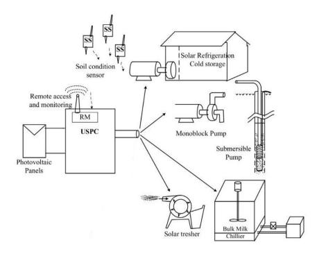
Fig. 1. USPC operation schematic diagram.
